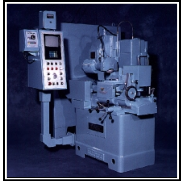
Modernized Heald Model 161 Rotary Surface Grinder modernized with PLC control of wheelslide (Level II scope of work, as described below).
